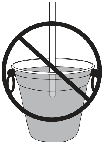
WRONG: Drain line is under water
