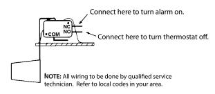
Safety switch: The safety overflow switch should be connected to a class II low voltage circuit. To control a thermostatic circuit the COM and NO connections from the safety switch are to be wired in series with the low voltage thermostat circuit to shut down the heating/AC circuit. The COM and NC switch contacts
