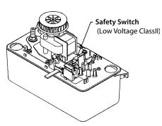
may be used to actuate a low voltage alarm circuit (connected in series) if the heating/cooling system can not be disrupted. The safety switch comes from the factory with leads connected to the COM and NO switch terminals. Typical hook-up of "NC" circuits would be (Figures 2 & 3).
