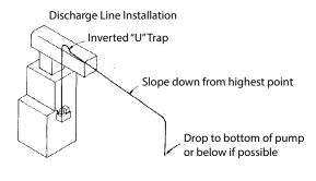
The outlet piping should be flexible tubing secured with a hose clamp (not provided) or pipe (3/8 inch I.D. maximum to prevent excessive flow back to unit). From condensate unit, extend discharge piping straight up as high as necessary. Do not extend this line above the head/GPH of the particular model being installed. From this high point, slope discharge line down slightly to a point above drain area; then turn down and extend
