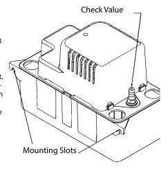
to a point below or approximately level with the bottom of the condensate unit. This will give a siphoning effect which will improve efficiency of the condensate unit and will, in most cases, eliminate the need for a check valve (Figure 5). If it is not possible to slope discharge line down, make an inverted "U" trap directly above the pump at the highest point.
