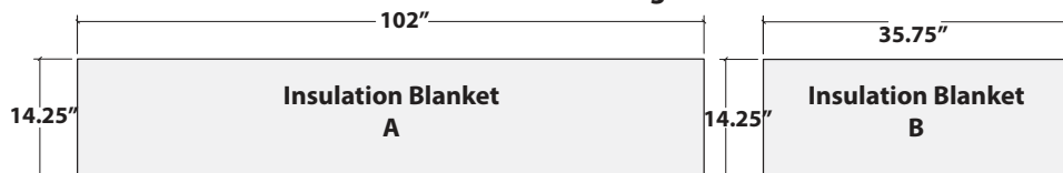
Ceiling Mount blanket dimensions
