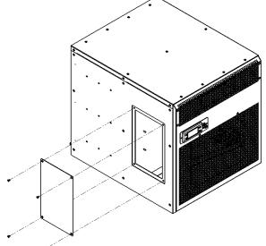
Remove the (4) screws and side access panel to view internal drip tray.
